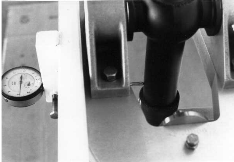
Photo #13: Reading poundage pull on hub.
